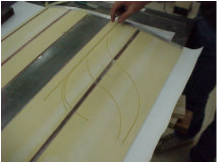
Figure 10 Third-Scale Model Construction: Routing Pressure Tubes
